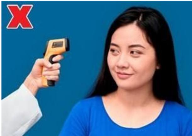
Figure 2: Incorrect Use – Not perpendicular to forehead
